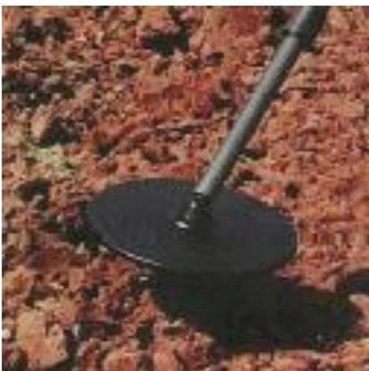
The detector design allows use both with and without earphone. The equipment has volume control facility. Detector gives detection sound when operated without earphone. If earphone is used the detection sound does not be heard, but only in earphone. The detector has a power control and sensitivity control to detect all type of ferrous/nonferrous metal. The detector have a visual display (led's) on the control unit to indicate detection and proximity of target metal. The led's are bright.
